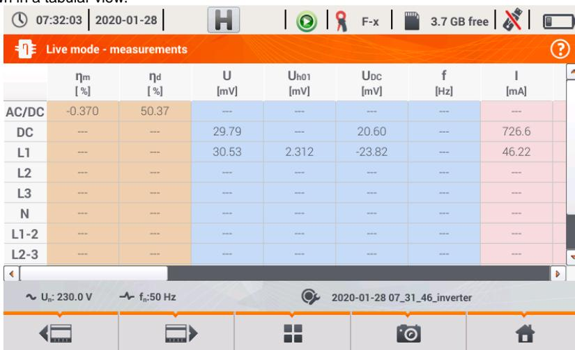
**Fig. 47. Live mode in tabular view for the inverter efficiency measurement mode.**
