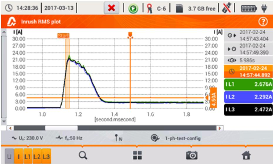
Fig. 43. Inrush current analysis – Inrush RMS plot.
