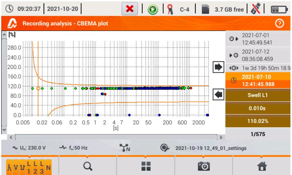
Fig. 32. Recording analysis - CBEMA graph.
