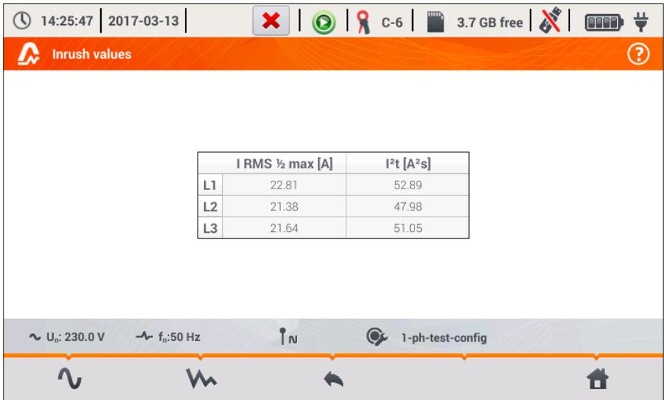
Fig. 44. Inrush current - characteristic parameters.
