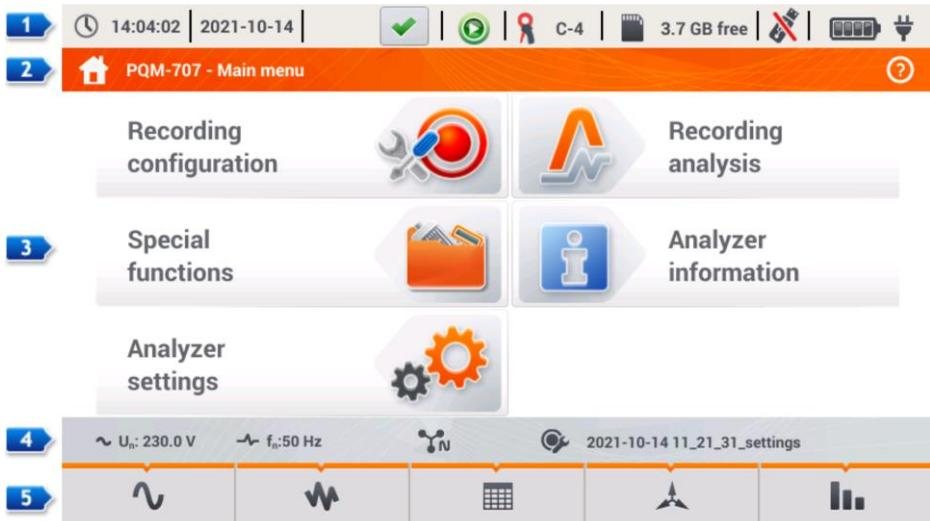
Fig. 2. Main elements of the analyzer screen.
