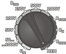
Set the rotary switch of function selection at **MEM** position.
