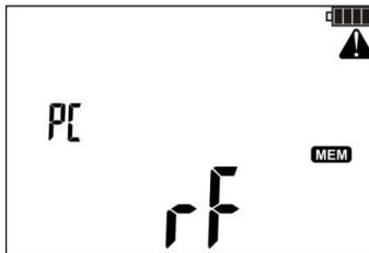
Press **ESC** to exit the transmission mode.
