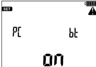
The meter displays the screen of wireless communication.
