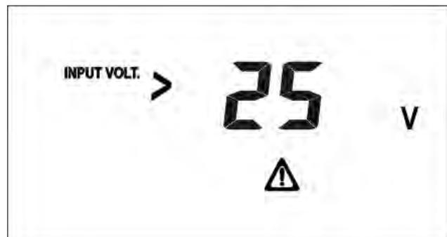
2. If, upon pressing the **START/STOP** key (with nominal test voltage set to  $\leq 1000V$  and load resistance  $\geq 5M\Omega$ ), the capacitance at input leads -Rx, +Rx is  $>$  allowable limit capacitance, the instrument gives a long acoustic signal and displays the screen reported here to the side for 3 seconds. Afterwards, the instrument returns to the initial screen.
