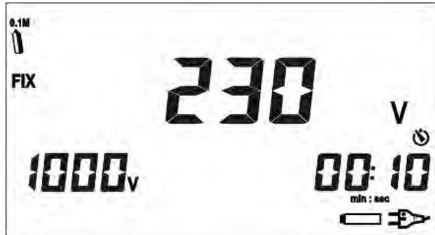
5. Press the **MODE/CLEAR SMOOTH** key to set one of the following test voltages: 250V, 500V, 1000V, 2500V, 5000V
