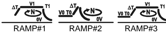
For each type of ramp, it is possible to set the duration, the test voltage and the number of times the ramp is repeated (§ 5.4.1, § 5.4.2, § 5.4.3).
