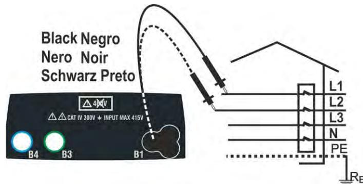
Fig. 32: Phase sequence check with test leads
