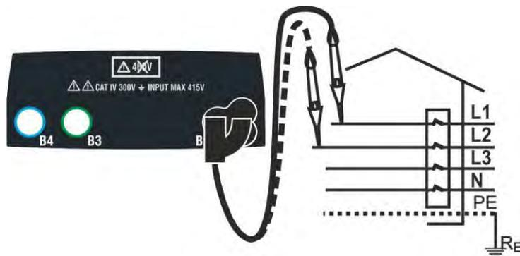
Fig. 33: Phase sequence check with remote switch probe
