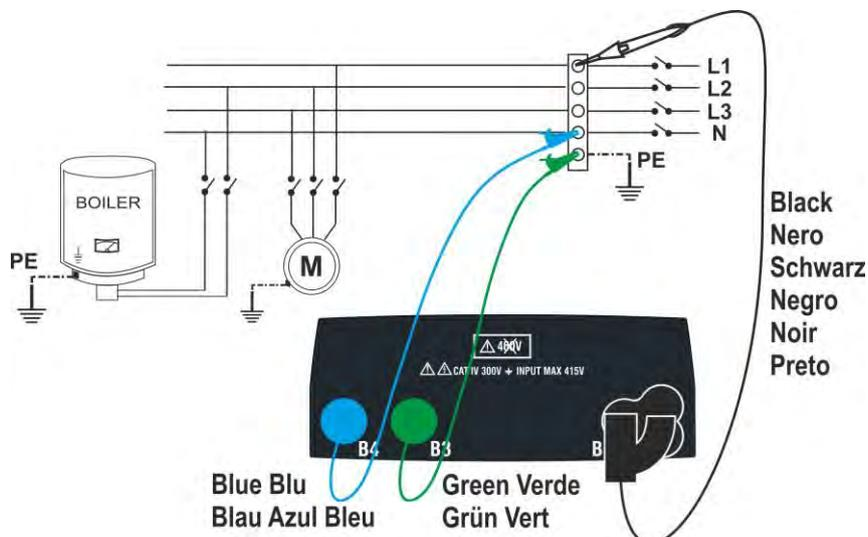
Fig. 12: Insulation between L-N-PE with single cables and remote switch probe (MAN and AUTO)
