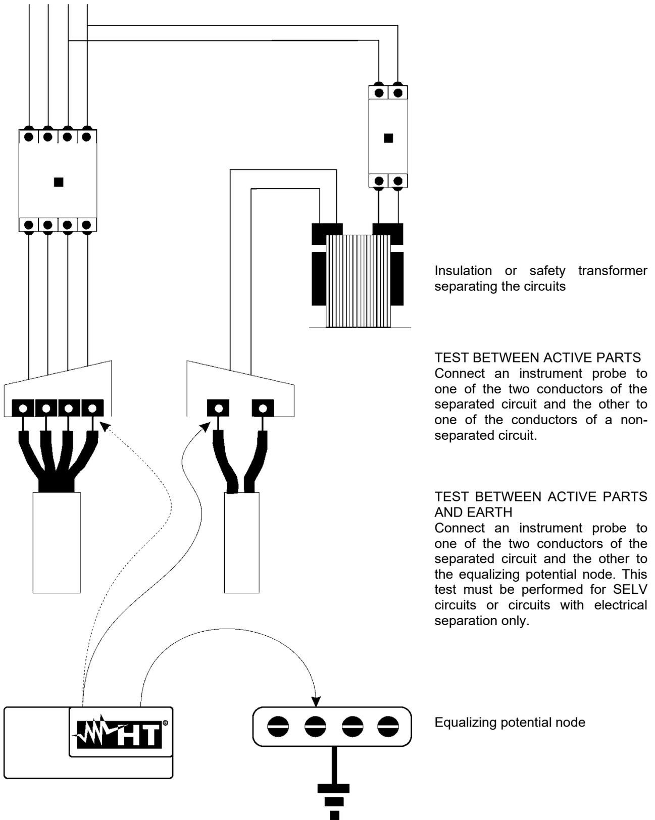
Fig. 37: Separation measurements between the circuits of a system
