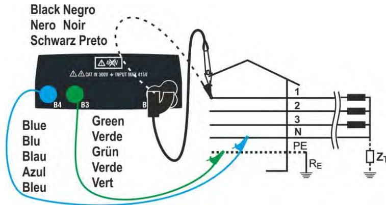
Fig. 28: P-PE measurement for IT systems by means of single cables and remote probe
