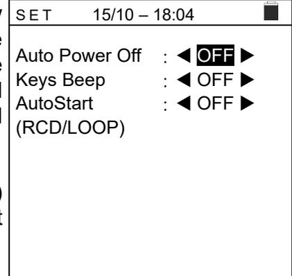
Select the desired option by means of the arrow keys (▲,▼) and (◀, ▶). To store settings, press the **ENTER** key, to quit without confirming the changes made, press the **ESC** key
