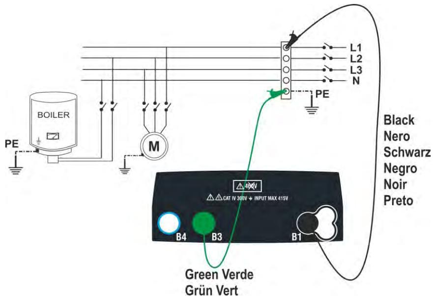
Fig. 15: Insulation between L-PE by means of single cables (TMR mode)
