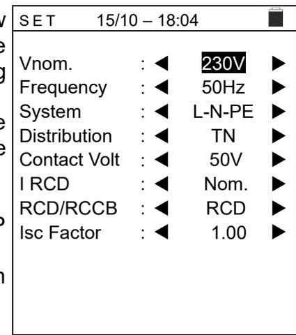
Select the desired option by means of the arrow keys (▲,▼). To store settings, press the **ENTER** key, to quit without confirming the changes made, press the **ESC** key
