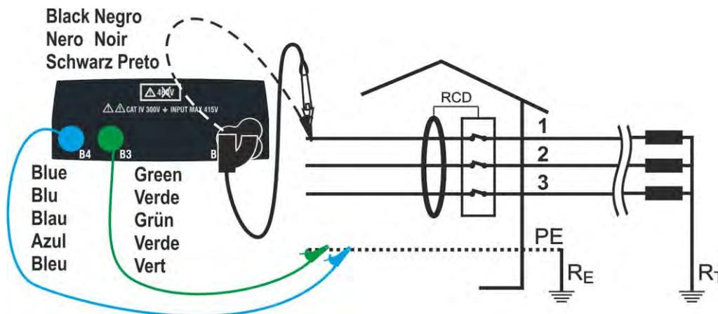
Fig. 22: Connection for a 400V + PE (no N) system with cables and remote switch probe
