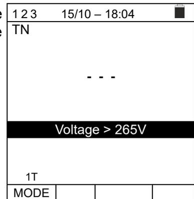
3. If, between the test start and the acquisition of the first voltage or between the acquisition of the first and second voltage, a time longer than approx. 10s has elapsed, the instrument displays a screen like the one to the side. It is necessary to repeat the test.
