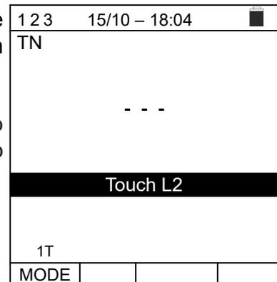
6. The instrument gives out a long sound until input voltage is present. At the end of the test, if the detected phase sequence is correct, the instrument displays a screen like the one shown to the side (result "**123**") and the "**OK**" message.
