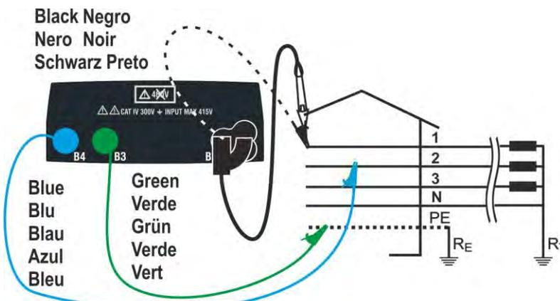
Fig. 26: P-P measurement for 400V+N+PE three-phase systems
