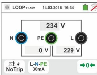
5. Press the **GO/STOP** key **for few seconds** or the **START** key on the remote lead. During this whole stage, do not disconnect the measuring leads of the instrument from the system under test.
