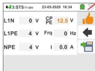
Press the **SAVE** key or touch the icon for the partial saving of the test and follows with the next test of **E fault simulation** (point 43)
