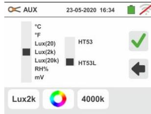
4. **In case of LED/colored sources** it is necessary to set the correspondent **color temperature** value (expressed in K) in the range: **2500K ÷ 6500K** in order to have a correct measurement result
