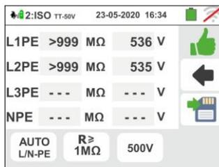
Press the **SAVE** key or touch the icon for the partial saving of the test and continue with the next test on L3 phase. The followed screen is shown on the display
