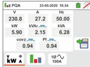
6. The screen to the side shows the real time values of electrical parameters in a Three phase balanced plant. For the meaning of the parameters refer to § 13.15. The symbols “**m**” and “**+**” show the type Inductive or Capacitive of the load respectively.
