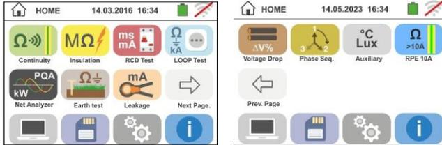
Fig. 5: General menu of the instrument
