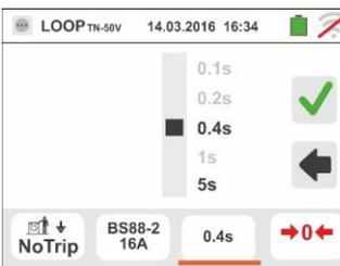
6. If possible, disconnect all loads connected downstream of the measured point, as the impedance of these users could distort the test results. Perform the preliminary calibration of the test leads as described in § 6.4.2 Connect the alligator clips or the remote lead to the electrical mains according to Fig. 18, Fig. 19, Fig. 20 and Fig. 22 in the farthest possible point respect the protection on test.
