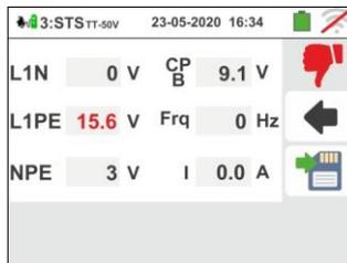
Press the **SAVE** key or touch the icon for the partial saving of the test and to **end the test sequence**. The instrument shows the message shown in the followed screen for a few seconds
