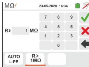
Touch the icon to zero the value in the "R≥" field. Use the virtual keyboard to set the value between **0.01MΩ** and **999MΩ**.
