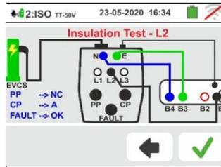
16 The measurement result of the **L2PE test** is shown in the screen to the side. The values of the real test voltages are shown on the display
