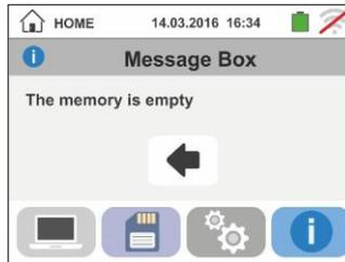
2. In case tries to define a new sub-node over the 3rd level the instrument provides the warning screen shown to the side and blocks the operation
