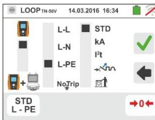
3. If possible, disconnect all loads connected downstream of the measuring point, as the impedance of these users could distort the test results.
