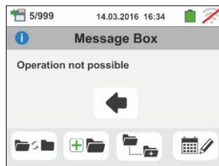
3. In case tries to create a sub-node by using a just used name, the instrument provides the warning screen shown to the side and is necessary to define a new name
