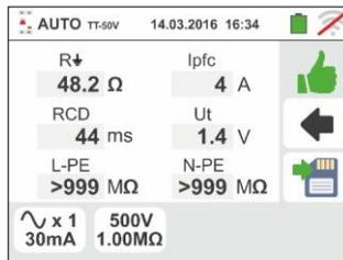
9. In case of **positive** result of the three test sequentially performed as **NoTrip** (see § 13.8), **RCD** (see § 13.4) and **MΩ L/N-PE** the symbol is shown and the screen to the side is displayed by the instrument.
