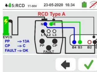
57 The test is performed by the instrument considering only General RCD of STD (G) type, type A/F and in Ramp mode (📈) 0°. Touch the second icon. The followed screen is shown on the display
