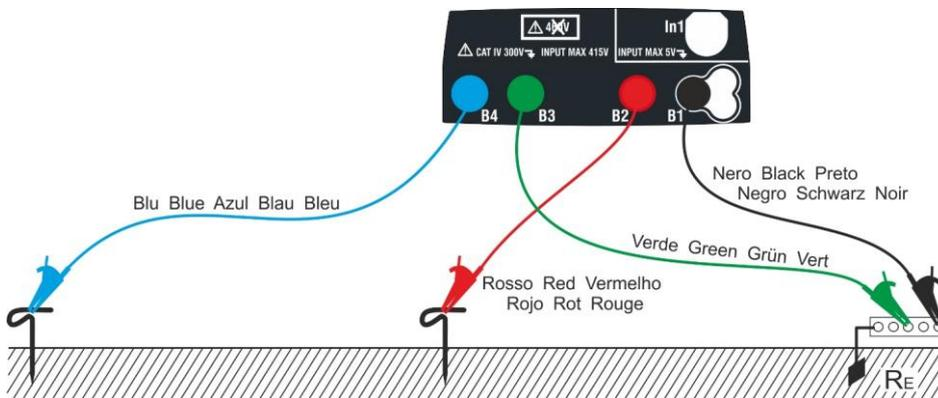
Fig. 28: Three-wire earth resistance measurement
