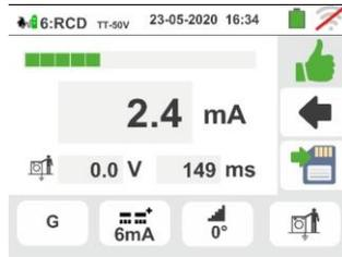
Press the **SAVE** key or touch the icon
