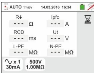
7. Press the **GO/STOP** key **for few seconds** or the **START** key on the remote lead. During this whole stage, do not disconnect the measuring leads of the instrument from the system under test. In case of **RCD tripping current measurement** selection the screen to the side appears on the display when the hourglass icon indicates the performance of the test
