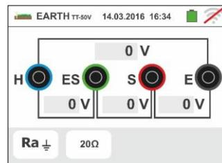
5. Touch the icon to zero the value in the "Ω" field and use the virtual keyboard to set the value of limit earth resistance between **1Ω** and **999Ω**. Confirm the choice by going back to the initial measurement screen.
