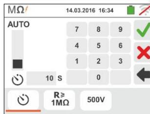
4. Touch the icon "R≥xxΩ" to set the minimum limit value of the insulation resistance on which the instrument makes the comparison with the measured value. The screen to the side appears on the display.
