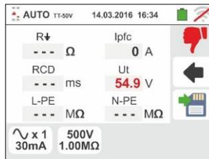
11 In case of **negative** result of the **RCDX1**, the auto test is automatically blocked, the symbol is shown and the screen to the side is displayed. Note red value of the tripping time
