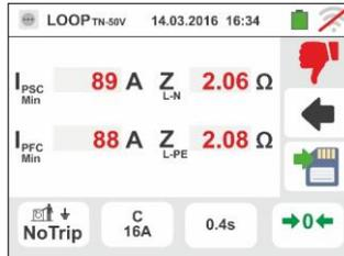
9. If the electrical Noise between N and PE conductors is so high that it could compromise the result accuracy, the symbol
