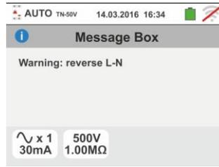
7. If the instrument detects that the phase and PE leads are inverted, it does not carry out the test and a screen similar to the one reported to the side is displayed. Check the connection of measuring cables
