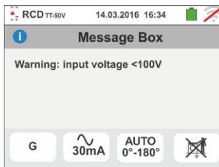
3. If the instrument detects the absence of the signal to terminal B1 (phase conductor), it provides the warning screen shown to the side and blocks the execution of the tests.
