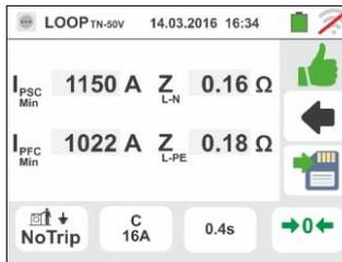
8. (**Z<sub>L-PE</sub> HIGHER to limit impedance relative to protection device within the specified time** – see § 13.7), the screen to the side is displayed by the instrument. Press the **SAVE** button or touch the
