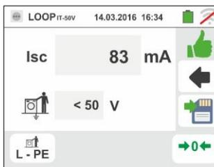
5. In case of negative result (contact voltage at the point >50V or >25V), the screen to the side is displayed by the instrument.
