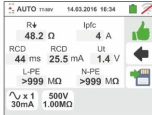
10 In case of **negative** result of the **NoTrip**, the auto test is automatically blocked, the symbol is shown and the screen to the side is displayed. Note red value of the contact voltage
