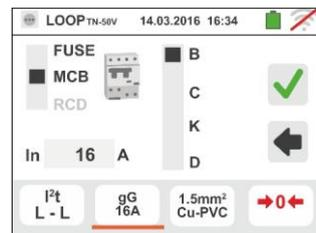
4. Touch the icon to zero the value in the In field and use the virtual keyboard to set the value of the RCD rated current within the values allowed by the instrument.
