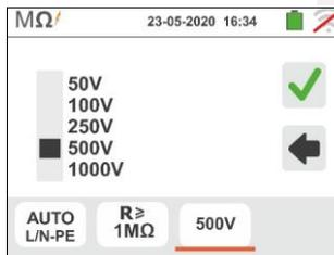
Move the slide bar reference to the desired value for test voltage by choosing among **50, 100, 250, 500, 1000VDC**. Confirm the choice by going back to the initial measurement screen. Note the presence of the set limit value.
