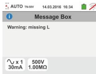
4. If the instrument detects the absence of the signal to terminal B4 (neutral conductor), it provides the warning screen shown to the side and blocks the execution of the tests
