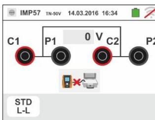
4. The symbol indicates the correct connection and recognition of the IMP57 by the instrument. Check the green STATUS LED lighting on the IMP57.
