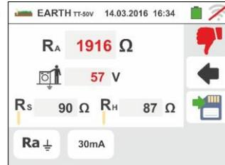
8. For **earth resistance measurement in IT systems**, in case of **negative** result (see § 13.9), the screen to the side is displayed by the instrument. It contains the value of contact voltage in the secondary display, the value of contact resistance of the voltage probe ( $R_s$ ) and the value of contact resistance of the current probe ( $R_h$ ).
