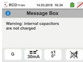
14 **For only RCD type B/B+** if the instrument detects a input voltage  $V_{L-N} < 190V$ , it provides the warning screen shown to the side and blocks the test. Check the values of the voltages on the installation
