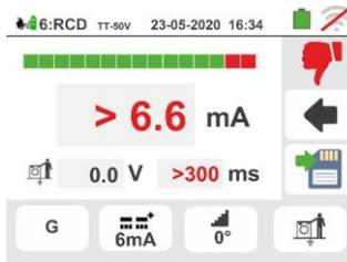
Press the **SAVE** key or touch the icon
