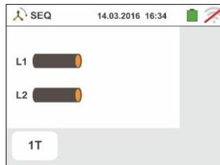
2. Move the slide bar reference in the position "1T" for the selection of the test with 1 terminal or in the position "2T" for the selection of the test with 2 terminals.
