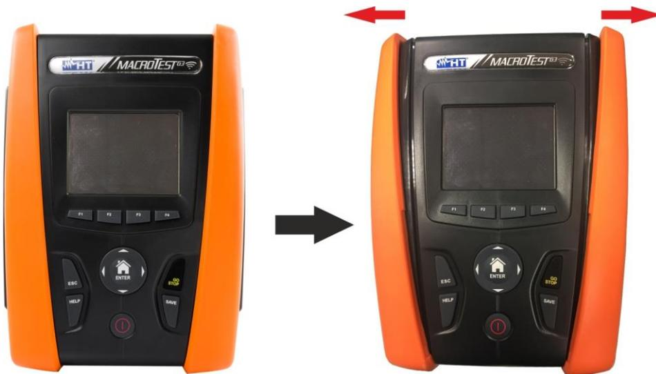
Fig. 40: Remove lateral half-shells
