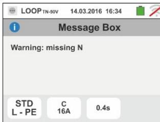
5. If the instrument detects the absence of the signal to terminal B3 (PE conductor), it provides the warning screen shown to the side and blocks the execution of the tests.
