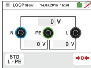
2. Move the left slide bar reference by selecting the icon to execute the measurement only with the instrument or the icon to execute the measurement with the instrument + optional accessory IMP57 (see § 6.4.13). Move the central slide bar reference by selecting the "L-L, L-N or L-PE" options. Move the right slide bar reference by selecting the "STD" option. Confirm the choice by going back to the previous screen.
