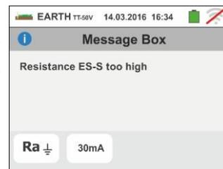
3. When starting a measurement, the instrument checks the continuity of measuring cables. **If the ampermetric circuit (blue cable H and black cable E) is interrupted or its resistance value is too high**, the instrument displays a screen similar to the one on the side.
