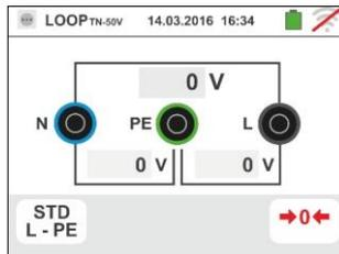
2. Touch the icon in order to select the test leads calibration or the icon to select the cable with Shuko plug calibration as shown in the following screen
