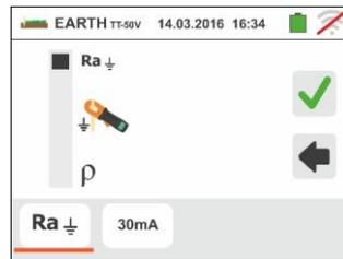
Touch the second icon in the lower left corner to set the tripping current of the differential switch (**TT and IT systems**). The following screen appears on the display:
