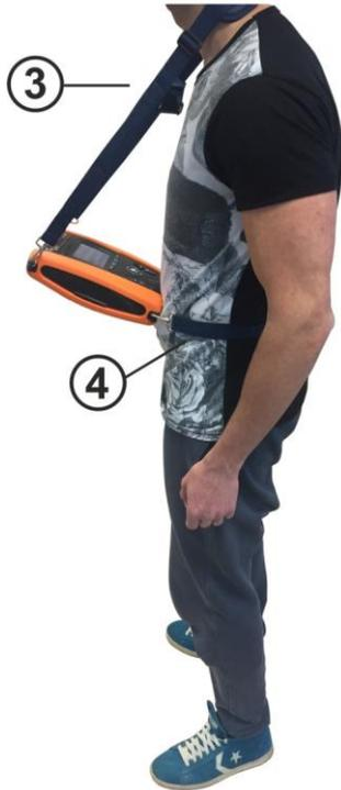
Fig. 43: Complete mounting of set strap
