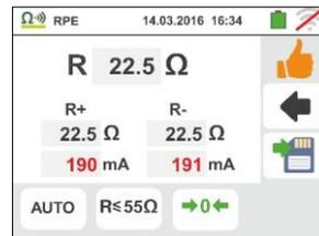
2. If in '→ 0 ←' mode the instrument detects a resistance higher than 5Ω at its terminals, it resets the offset value and displays a screen like the one to the side. The '→ 0 ←' icon is shown on the display to indicate the calibration reset value (i.e. performing the operation with open terminals).
