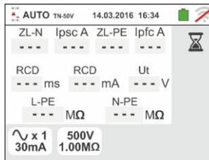
8. In case of **positive** result of the three test sequentially performed as **NoTrip** (ZL-N and ZL-PE<199Ω), **RCDX1** (see § 13.4) and **MΩ L/N-PE** the symbol is shown and the screen to the side is displayed by the instrument
