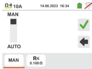
4. Touch the icon to reset the value in the "Ω" field and use the virtual keyboard to set the value of the maximum limit resistance used by the instrument for evaluating the continuity test in the field: **0.003Ω ÷ 0.500Ω** in steps of **0.001Ω**. Confirm your choice by returning to the previous screen
