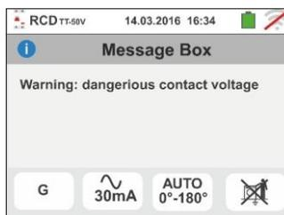
11 If the instrument detects a voltage  $V_{n-pe} > 50V$  (or the analogue  $V_{n-pe} > 25V$ ) it provides the warning screen shown to the side and blocks the test for safety reasons. Check the PE conductor and earth plant efficiency
