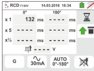
13 At the end of the test, if the tripping time of a test does not comply with what is indicated in Table 6 (see § 13.4).
