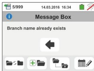
4. In case tries to define a numebr of nodes of 1st, 2nd and 3rd level higher than 250 (for each level), the instrument provides the warning screen shown to the side
