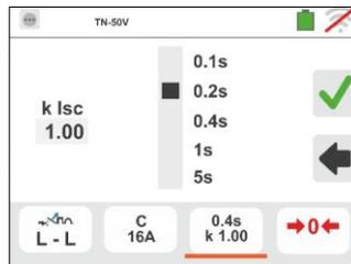
6. Touch the icon to zero the value in the field and use the virtual keyboard to set the calculation coefficient of the short circuit current **Isc** within the values allowed by the instrument
