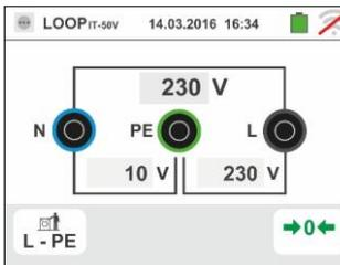
4. Press the **GO/STOP** key for few seconds or the **START** key on the remote lead. During this whole stage, do not disconnect the measuring leads of the instrument from the system under test.
