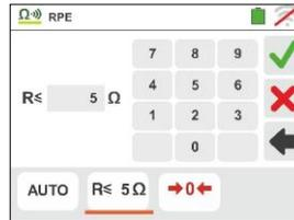
Touch the icon to zero the value in the "R≤" field. Use the virtual keyboard to set the value between **0.01Ω** and **9.99Ω**. Confirm the choice by going back to the initial measurement screen. Note the presence of the set limit value.
