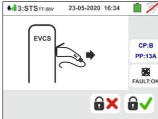
Press the icon if the operation is successful and continue with the next test (point 27) or press the icon to **end the test sequence**
