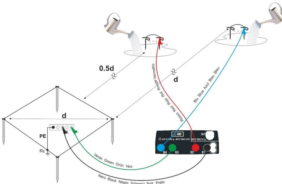
Fig. 48: Ground measurement for big-sized earth networks
