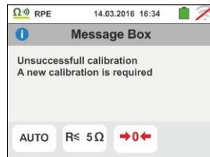
3. In case the instrument detects a calibration reset (performing the operation with open terminals), it gives out a long sound and displays a screen like the one to the side. The '→ 0 ←' icon is shown on the display to indicate the calibration reset value.
