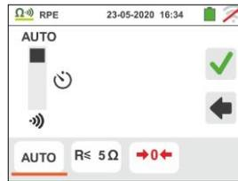
3. Touch the icon to zero the value in the Timer field and use the virtual keyboard to set the value in seconds between **1s** and **15s**. Confirm the choice by going back to the initial measurement screen.
