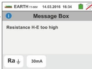
4. When starting a measurement, the instrument checks the situation of B2 (S) and B3 (ES) inputs. In case of reverse of conductors on the installation it blocks the test and the message is shown
