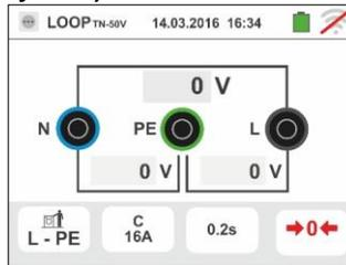
2. Move the left slide bar reference by selecting the icon to execute the measurement.
