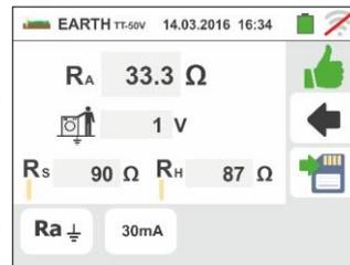
7. For **earth resistance measurement in TT systems**, in case of **negative** result (see § 13.7), the screen to the side is displayed by the instrument. It contains the value of contact voltage in the secondary display, the value of contact resistance of the voltage probe ( $R_s$ ) and the value of contact resistance of the current probe ( $R_h$ ). Note the presence of the measurement result highlighted in red.
