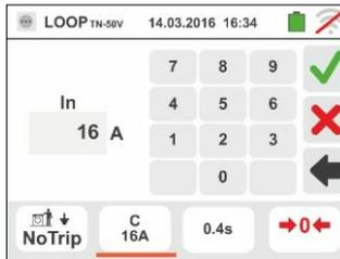
5. Move the slide bar reference by selecting the protection tripping time between the options: **0.1s**, **0.2s**, **0.4s**, **1s**, **5s** (all countries except AUS/NZ), **0.4s**, **5s** (Fuse protection for AUS/NZ) and **0.4s** (MCB protection for AUS/NZ)
