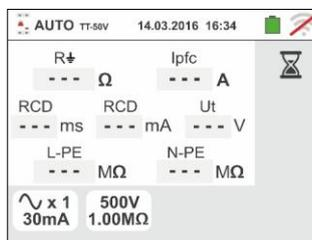
8. In case of **positive** result of the three test sequentially performed as **NoTrip** (see § 13.8), **RCDX1** (see § 13.4) and **MΩ L/N-PE** the symbol is shown and the screen to the side is displayed by the instrument
