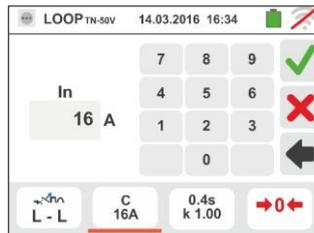
5. Move the slide bar reference by selecting the protection tripping time between the options: **0.1s, 0.2s, 0.4s, 1s, 5s**. Confirm the choice by going back to the initial measurement screen.
