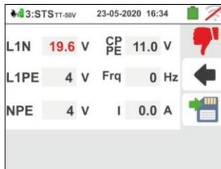
Press the **SAVE** key or touch the icon for the partial saving of the test and to **end the test sequence**. The instrument shows the message shown in the followed screen for a few seconds
