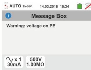
10. If the instrument detects a dangerous contact voltage  $U_t$  (over the set limit 25V or 50V) in the starting pre-test, it provides the warning screen shown to the side and blocks the execution of the tests. Check the PE conductor and earth plant efficiency
