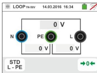
6. The value of the test leads/Shuko plug resistance various plugs is maintained by the instrument up to the reset operation performed by the user (for example for the insertion of cables with different lengths). To perform the reset of saved calibration value, touch the icon. The screen to the side appears on the display
