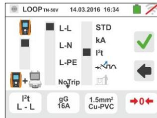
3. Move the slide bar reference by selecting the type of protection (Fuse of type **gG** or **aM** or magnetothermal MCB in curve **B**, **C**, **K**, **D**).
