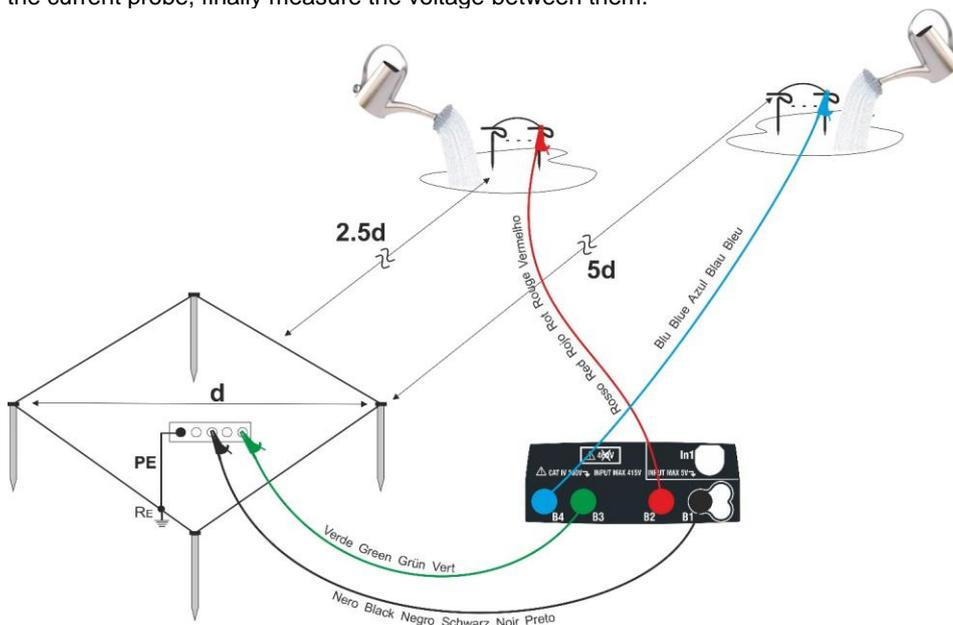
Fig. 47: Ground measurement for small-sized earth networks
