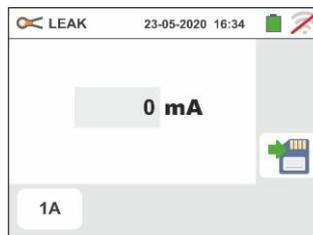
2. Touch the
