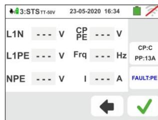
40 The result of the measurement is shown in the screen to the side. The symbol indicates the correct result of the measurement. The symbol also indicates a positive result of the measurement but with values outside the limits present in the Table 4
