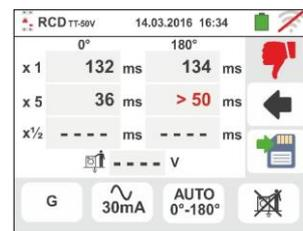
11 The test has a positive result if all tripping times of **molded case type STD** comply with what indicated in Table 6 (see § 13.4). The test has a negative result when one of the values is out of range. During this whole stage, do not disconnect the measuring leads of the instrument from the system on test.
