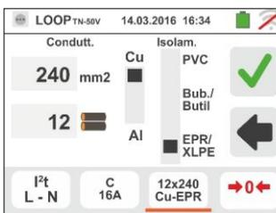
Move the central slide bar reference by selecting the type of conductor. The available options are **Cu** (Copper) and **Al** (Aluminum).
