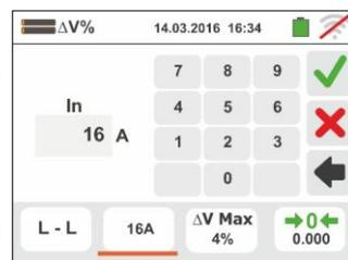
5. Touch the icon
