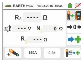
Rods resistance measurement with clamp T2100 connected to the instrument
