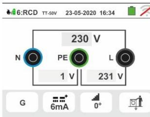
66 Move the third slide bar reference by selecting the desired rated current of the differential switch between the options: **6,10, 30, 100, 300mA (type B/B+) or 6mA (type DD)**
