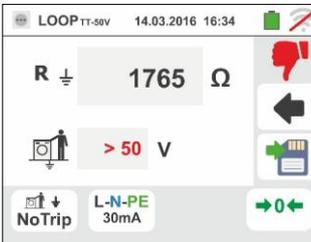
Press the **SAVE** button or touch the
