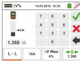
4. Touch the icon to zero the value in “A” field and use the virtual keyboard to set the value of rated current of protection device in the range **1A** to **9999A**. Confirm selection and go back to the previous screen.
