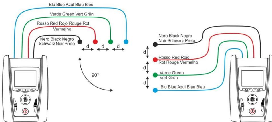
Fig. 49: Ground resistivity measurement
