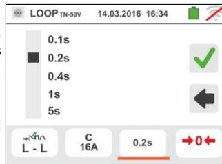
6. If possible, disconnect all loads connected downstream of the measured point, as the impedance of these users could distort the test results. Perform the preliminary calibration of the test leads as described in § 6.4.2 Connect the shuko plug, the alligator clips or the remote lead to the electrical mains according to Fig. 18, Fig. 19, Fig. 20 and Fig. 22 in the farthest possible point respect the protection on test
