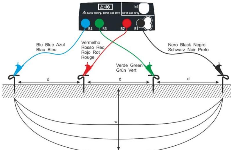
Fig. 31: Soil resistivity measurement
