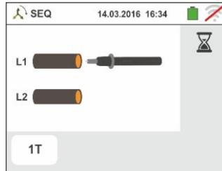
5. Once the correct voltage recognized, the ⚡ symbol is shown on the display. The instrument gives out a long sound until input voltage is present.
