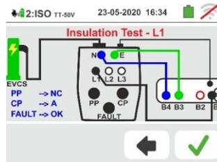
Press the icon to continue with the test or press the icon to exit the test and return to the initial screen
