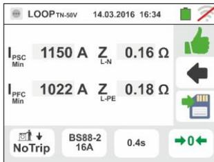
8. (**Z<sub>L-PE</sub> OR Z<sub>L-N</sub> HIGHER to limit impedance relative to protection device within the specified time** – see § 13.7), the screen to the side is displayed by the instrument. Press the **SAVE** button or touch the
