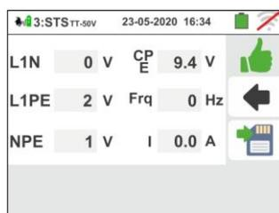
Press the **SAVE** key or touch the icon to end the status control test and save the final result in the instrument's memory (see § 7.1)
