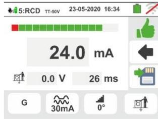
Press the **SAVE** key or touch the icon for the partial saving of the test. The instrument shows the message shown in the followed screen for a few seconds
