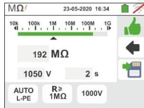
11. At the end of the test, if the value of the measured resistance is lower than the set limit, the screen to the side is shown on the display.
