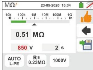
7. **In the L/N-PE test** if in one of both test the instrument measures a resistance higher than the set limit value but for which it is not able to generate the rated voltage, the screen to the side is displayed.
