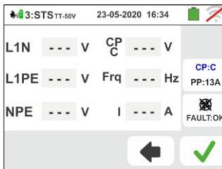
Press the icon to activate the **test on C state**. The following screen is shown on the display
