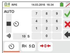
4. Touch the icon " $R \leq x\Omega$ " to set the maximum limit value of the resistance on which the instrument makes the comparison with the measured value. The screen to the side appears on the display.
