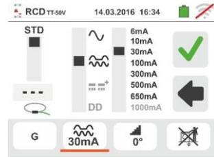
59 Ramp mode (📈) is fixed on the instrument. Move the reference of the lower sliding bar by selecting the type of display of the tripping current during the ramp test between the "NOM" or "REAL" options (see § 6.3)
