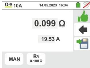
7. At the end of the test, if the measured resistance value is higher than the set limit, the screen to the side is shown on the display. The value is shown in red and the
