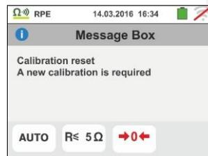
4. If the instrument detects a calibrated resistance higher than measured resistance (e.g. by using test cables different from the supplied ones) at its terminals, it gives out a long sound and displays a screen like the one to the side. Perform a calibration reset with open terminals and start a new calibration.
