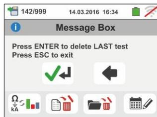
5. Touch the icon to delete **all the results stored in the memory of the instrument**. The following screen appears on the display:
