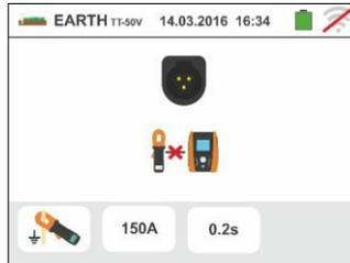
2. Connect the clamp T2100 by inserting the connector into input **In1** of the instrument. Turn the clamp on and put it in "RS232" mode (see the user manual of the clamp). The **232<sup>5</sup>** symbol appears on the display of the clamp. **In these conditions, the instrument-clamp group is ready to perform the measurements.** The following screen is shown on the display by the instrument.
