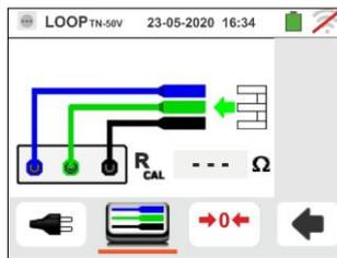
3. Insert the **ZEROLOOP** metallic accessory into the three banana connectors of the measurement cables (L-N-PE) or into the metal connectors of the Shuko plug (differently in the various types depending on the country of use) as shown in the following
