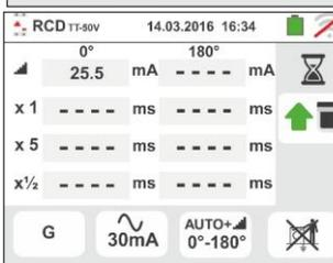
**NOTE: the value of contact voltage is not shows in this test**
