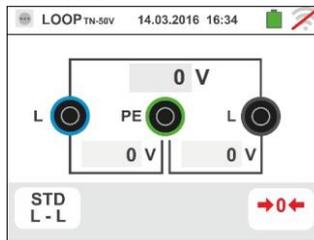
2. Move the left slide bar reference by selecting the icon to execute the measurement only with the instrument or the icon to execute the measurement with the instrument + optional accessory IMP57 (see § 6.4.13). Move the central slide bar reference by selecting the "L-L", "L-N" or "L-PE" options (for TN systems only). Move the right slide bar reference by selecting the "kA" option.
