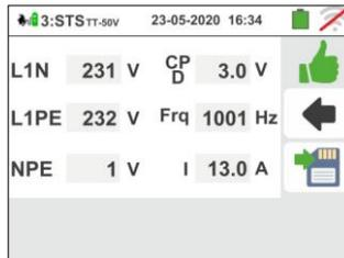
Press the **SAVE** key or touch the icon for the partial saving of the test and follows with the next test **of PE fault simulation** (point 39)
