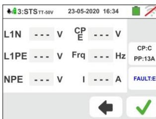
**NOTE: Some EVSE stations could not manage this error condition. In this case, leave the Fault selector in the PE position to perform the test**
