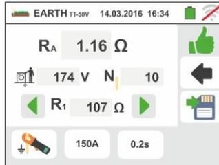
In case of positive result (see § 13.7 and § 13.12), the instrument shows the symbol and it is also possible to scroll through the values of partial resistances by touching the keys and .
