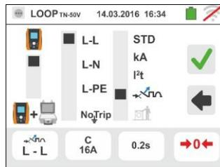
Move the central slide bar reference by selecting the “L-L”, “L-N” or “L-PE” options (for TN systems only).
