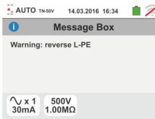
8. If the differential switch being tested trips during the preliminary checks (performed automatically by the instrument before executing the selected test), the instrument does not carry out the test and displays a screen like the one to the side. Check that the IdN set value is consistent with the differential switch in question and that all loads connected downstream of it are disconnected
