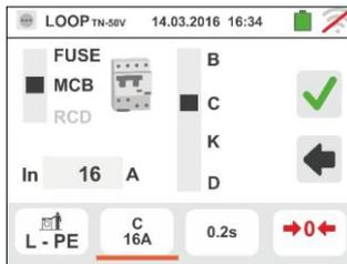
4. Touch the icon to zero the value in the In field and use the virtual keyboard to set the value of the nominal current of the protection within the values allowed by the instrument (see § 6.4.5)
