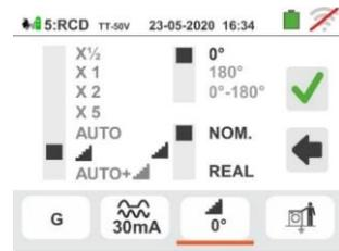
60 During this whole phase, do not disconnect the measuring terminals of the instrument from the system. At the end of the test, if the tripping current is within the values of the table in the relevant § 11.1 the instrument
