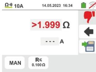
8. **In the AUTO measurement**, the instrument **goes into standby** and displays the screen to the side after performed a test. **Disconnect the test leads and connect them to the next test point to trigger the new measurement**
