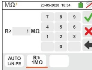
Touch the icon to zero the value in the "R≥" field. Use the virtual keyboard to set the value between **0.01MΩ** and **999MΩ**. Confirm the choice by going back to the initial measurement screen. Note the presence of the set limit value.
