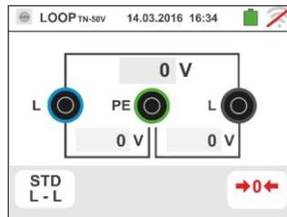
2. Move the left slide bar reference by selecting the icon to execute the measurement only with the instrument or the icon to execute the measurement with the instrument + optional accessory IMP57 (see § 6.4.13).
