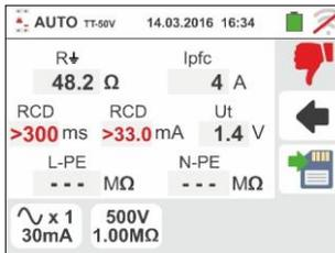
13 In case of **negative** result of the **MΩ L-PE**, the auto test is automatically blocked, the symbol is shown and the screen to the side is displayed. Note red value (lower than minimum set threshold) of the L-PE insulation resistance
