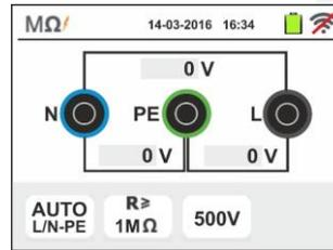
2. Move the slide bar reference in the positions "AUTO" (Automatic mode) or "⌚" (Timer mode). Move the right slide bar reference in the "L/N-PE" position. Confirm the choice by going back to the previous screen.
