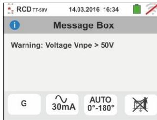
12 If the instrument detects in the input terminals a too high external impedance such that it can not provides the nominal current, it provides the warning screen shown to the side and blocks the test. Disconnect the possible loads downstream the LCD before perform the test
