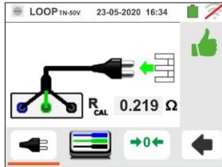
5. Touch the icon to back to the measurement main screen. Note the green icon which means the successful test leads calibration and proceed with the measurements described in the following paragraphs
