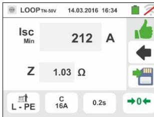
8. In case of negative result (calculated minimum short-circuit current **LOWER** than tripping current of the protection device within the specified time – see § 13.6), the screen to the side is displayed by the instrument
