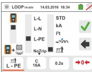
3. Move the slide bar reference by selecting the type of protection (Fuse of type **gG** or **aM** or magnetothermal MCB in curve **B, C, K, D**), (Fuse of type **BS88-2, BS88-3, BS3036, BS1362** or magnetothermal MCB in curve **B, C, D** – UK country). For **AUS/NZ** country magnetothermal MCB in curve **B, C, D**.
