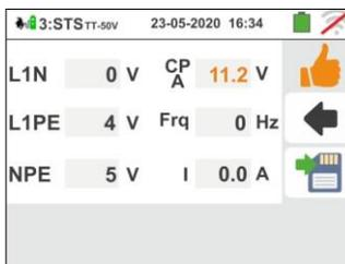
23 If the test fails, the screen like the one on the side is shown on the display. The incorrect value of the parameter is shown in red and the symbol indicates the non-ok result of the measurement
