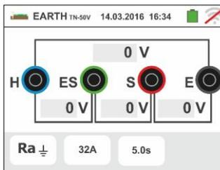
5. Touch the icon to zero the value in the "A" field and use the virtual keyboard to set the value of fault current (declared by the Energy distribution board) between **1A** and **9999A**. Confirm the choice by going back to the initial measurement screen.
