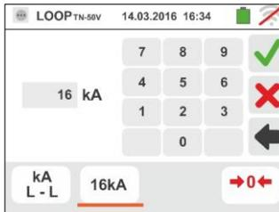
4. If possible, disconnect all loads connected downstream of the measured point, as the impedance of these users could distort the test results. Perform the preliminary calibration of the test leads as described in § 6.4.2 Connect the shuko plug, the alligator clips or the remote lead to the electrical mains according to Fig. 18, Fig. 19, Fig. 20 and Fig. 22 in the nearest possible point to the protection device
