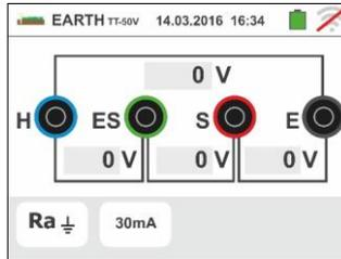
Touch the first icon in the lower left corner to set the measuring mode. The following screen appears on the display:
