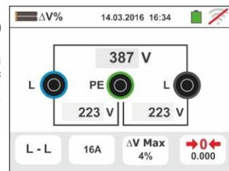
8. The value of **Z1 (Offset)** impedance is shown on the display and is automatically included on the lower right icon, together with the “
