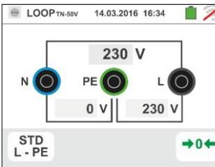
6. The value of the assumed short-circuit current (Isc) is shown in the upper part of the display, while the Line/Loop Z<sub>PE</sub> impedance is shown at the bottom of the display. Press the **SAVE** button or touch the icon to save the measurement (see § 7.1).
