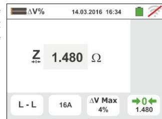
9. Connect the instrument to the final point of the main line being tested according to Fig. 34 or Fig. 35 in order to measure the **Z2** impedance at the end of line. The screen to the side is displayed. Note the previously measured Z1 (Offset) value displayed
