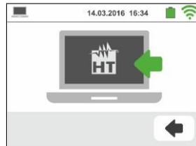
3. Launch the management software, select the "WiFi" port and "Detect instrument" within the section "PC-Instrument connection"
