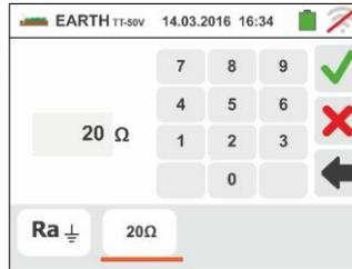
6. Press the **GO/STOP** key. During this whole stage, do not disconnect the measuring leads of the instrument from the system under test. The symbol is shown on the display for the entire duration of the test.
