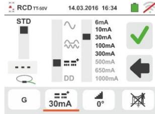
67 **Ramp mode (📈) is fixed on the instrument.** Move the reference of the lower sliding bar by selecting the type of display of the tripping current during the ramp test between the "**NOM**" or "**REAL**" options (see § 6.3).
