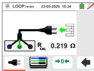
7. With open input terminals touch the icon. The “> 1Ω” indication is shown for a while in the **R<sub>CAL</sub>** field and the “Calibration Reset...” is shown at display.
