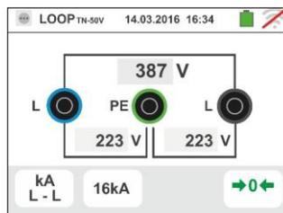
5. Press the **GO/STOP** key **for few seconds** or the **START** key on the remote lead. During this whole stage, do not disconnect the measuring leads of the instrument from the system under test.
