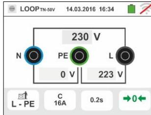
7. Press the **GO/STOP** key **for few seconds** or the **START** key on the remote lead. During this whole stage, do not disconnect the measuring leads of the instrument from the system under test.
