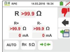
12. At the end of the test in the ")))" function if the value of the measured resistance is higher than the set limit, the value is shown in red. The indication ">1999Ω" indicates the overrange of the instrument as shown in the screen to the side
