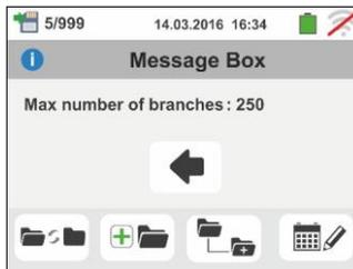
5. In case tries to include a comment of length higher than 30 chars, the instrument provides the warning screen shown to the side
