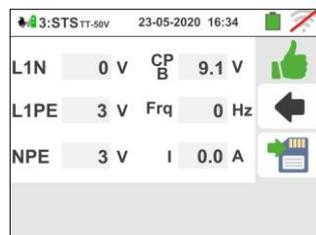
Press the **SAVE** key or touch the icon for the partial saving of the test and continue with the next test (point 31 to check C status or point 35 to check D status). Press again the **GO/STOP** key to repeat the test
