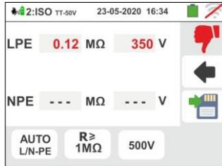
Press the **SAVE** key or touch the icon
