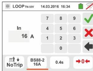
5. Move the slide bar reference by selecting the protection tripping time between the options: **0.4s**, **5s**
