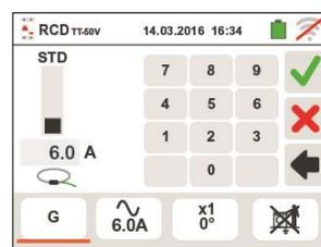
Move the second slide bar reference by selecting the waveform of the differential switch between the options: (type AC), (type A/F), (type B/B+), **DD** (type DD)
