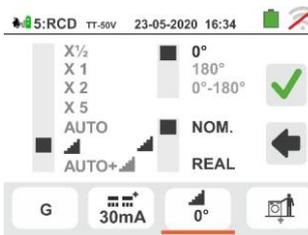
68 During this whole phase, do not disconnect the measuring terminals of the instrument from the system. At the end of the test, if the tripping current is within the values of the table in the relevant § 11.1 the instrument
