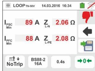
9. If the electrical Noise between N and PE conductors is so high that it could compromise the result accuracy, the symbol
