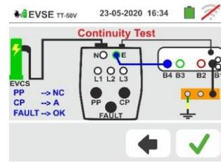
7. The RPE test is performed by the instrument **only in AUTO mode**. Set the limit threshold value and calibrate the measurement cables as shown in § 6.1
