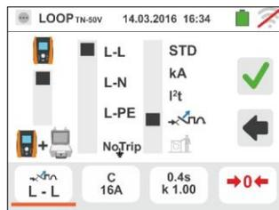
Touch the second icon to set the protection type and its rated current. The following screen appears on the display:
