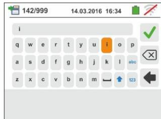
Further confirm to permanently save the measurement in the internal memory. A confirmation message is provided by the instrument.
