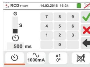
4. Move the left slide bar reference and select the type of RCD between the following options: **STD** (molded case RCD) and (earth leakage delay RCD with use of optional accessory RCDX10). In case of earth leakage relay RCD the following screen appears on the display
