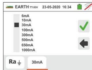
4. For **TN systems**, the instrument shows the initial screen as in the figure to the side.
