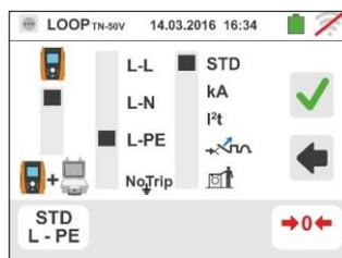
3. Touch the icon to zero the value in the kA field and use the virtual keyboard to set the value of the breaking capacity of the protection between **1kA** and **9999kA**
