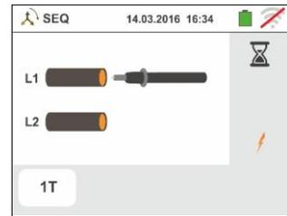
7. The symbol for the tip on phase L2 and the hourglass indicating the status of pending recognition of a voltage higher than the maximum allowed.
