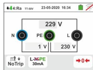
49 During this whole phase, do not disconnect the measuring terminals of the instrument from the system on test. In case of positive outcome (global earth resistance lower than the ratio between the limit contact voltage and the RCD tripping current - see § 13.8), the screen to the side is shown by the instrument in which the contact voltage value is indicated on the secondary display.
