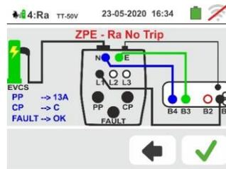
48 The test is performed by the instrument **only in "NoTrip" mode**. Refer to § 6.4.9 for the description on the setting of the test parameters relative to the trip out current of the RCD, **absence of neutral conductor (only possible measurement)** and the preliminary calibration of the measuring terminals
