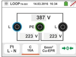
7. Press the **GO/STOP** key **for few seconds** or the **START** key on the remote lead. During this whole stage, do not disconnect the measuring leads of the instrument from the system under test.
