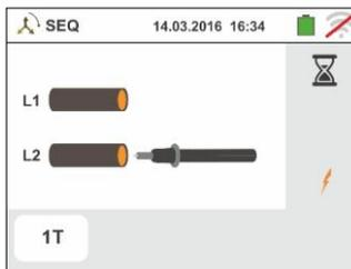
8. At the end of the test, if the detected phase sequence is correct, the instrument displays a screen like the one shown to the side (result "1-2-3").
