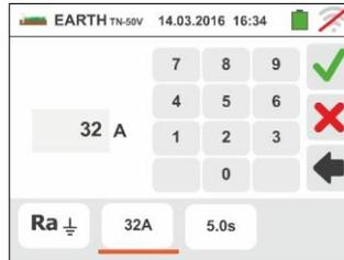
6. Touch the icon to zero the value in the "s" field and use the virtual keyboard to set the value of the time for fault elimination **t** (declared by the Energy distribution board) between **0.04s** and **10s**.
