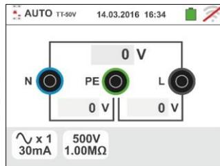
2. Move the left slide bar reference by selecting the waveform of the differential switch between the options:  $\sim$  (type AC),  $\sim$  (type A/F),  $\sim$  (type B/B+). Move the second slide bar reference by selecting the desired rated current of the differential switch between the options: **6mA, 10mA, 30mA, 100mA, 300mA**. Move the third slide bar reference by selecting the type of the test between the following options:
