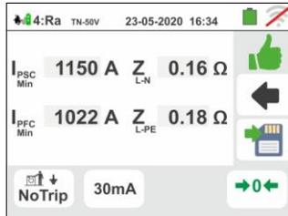
Press the **SAVE** key or touch the icon
