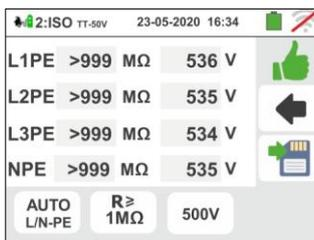
Press the **SAVE** key or touch the icon for the partial saving of the test and continue with the next test (point 21)
