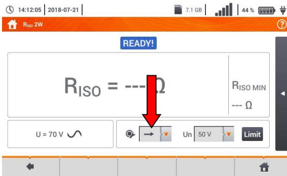
• Connect the meter probe or the adapter which the measurements will be performed with.
