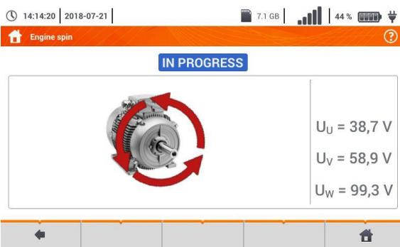
Arrows on the screen rotating **to the right** mean that the motor connected to a 3-phase network will rotate the shaft **to the right**.
