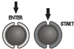
In order to maintain the measurement, press **ENTER** push-button while holding **START** push-button in the pressed position. In order to interrupt the measurement, press **START**.
