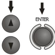
Use ▲, ▼ to select the distance between the probes, and press **ENTER** to trigger the measurement.
