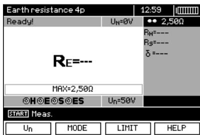
The meter is ready for measurement. Value of interference voltage  $U_n$  of the measured object may be read on the display.
