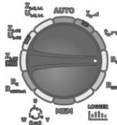
Turn the rotary switch to **R<sub>E</sub>** position.
