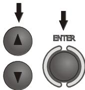
Use **▲**, **▼** to select the main result as  $Z_S$  impedance or as  $I_k$  - prospective short-circuit current and press **ENTER** to confirm your selection.
