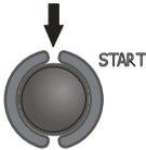
In order to start the next measurement without disconnecting test leads from the object, press **START**.
