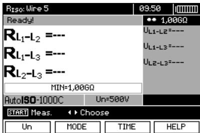
The meter is ready for measurement. Value of interference voltage can be read on the display.
