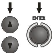
Use ▲ and ▼ select the measuring voltage, confirm by pressing **ENTER**.
