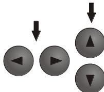
Use **◀**, **▶** to select the number of samples, then use **▲**, **▼** to set the number of samples - the recording time is calculated based on the sampling time and the number of samples. Press **F4** **OK** to enter the measurement screen.
