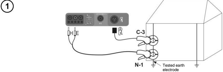
Transmitting clamps and measuring clamps should be attached to the tested earth electrode at a distance of at least 30 cm from each other. Connect transmitting clamps to **H** and **E** sockets, whereas the measuring clamps to the clamp socket.
