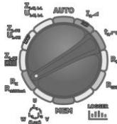
Set the rotary switch of function selection at  $R_x R_{\pm 200mA}$  position.
