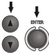
Use ▲, ▼ buttons to switch-off sound signals assigned to push buttons.
