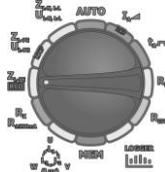
Set the rotary switch of function selection at ZL-PE **RCD** position.
