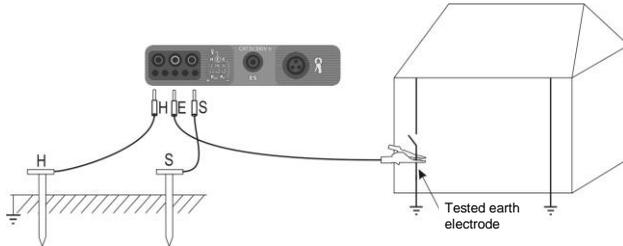
The current electrode (driven into earth) should be connected to **H** socket of the meter.
