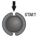
Press and hold **START** push-button. Measurement is performed continuously when the push-button is held in the pressed position.
