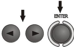
Use ◀ and ▶ to select deleting the measurements/recorder memory. Press **ENTER**-push-button.
