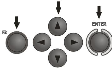
In order to set the security parameters press **F2**
