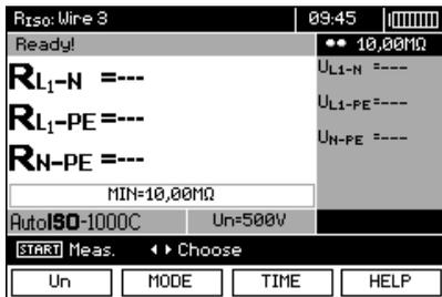
F1 ↓ Press **F1** **U<sub>N</sub>** push-button and move to selection of test voltage U<sub>N</sub>.
