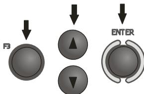
In order to select the voltage for calculating the prospective short circuit current I<sub>k</sub> - nominal or measured - press **F3**  I<sub>k</sub>.
