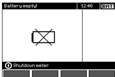
Batteries /rechargeable batteries are fully discharged, the measurement is stopped.
