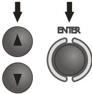
Use ▲ and ▼ to select desired position and press **ENTER** to confirm. For selecting the security means, use ◀ and ▶ to select the parameter and the use ▲ and ▼ to select its value.
