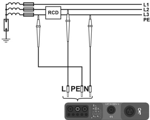
b) If there is a possibility of connecting PE channel of the meter before the RCD.
