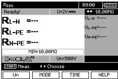
Press **F1** **U<sub>N</sub>** push-button and move to selection of test voltage U<sub>N</sub>.
