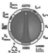
Set the rotary switch of function selection at **AUTO** position.
