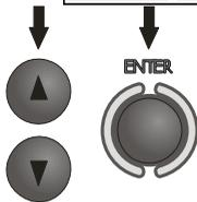
Use ▲ and ▼ to select the measuring voltage, confirm by pressing ENTER.
