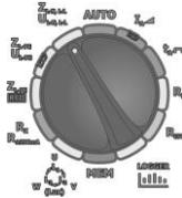
Set the rotary switch of function selection at  $Z_{L-N,L-L}/U_{L-N,L-L}$  position.
