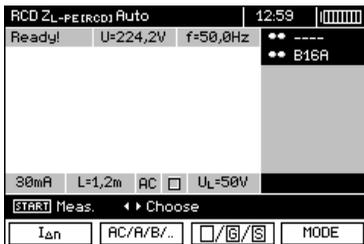
The meter is ready for measurement. Value of network voltage and frequency can be read on the display.
