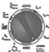
Set the rotary switch of function selection at **LOGGER** position.
