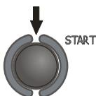
Press **START** push-button to start the measurement. If such measurements are selected that require triggering of RCD, operator of the meter should be in the vicinity of RCD and switch it on each time after it is triggered until the measurements are completed (a longer interruption may signify completion of the measurements).
