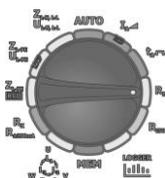
Set the rotary switch of function selection at **RE** position.
