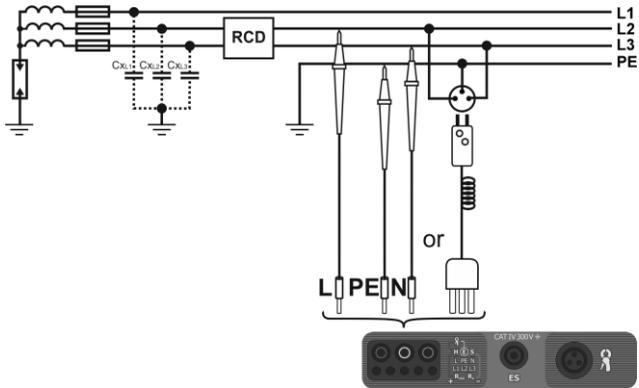
a) Parasitic capacitance is used during the measurement.
