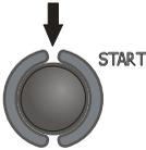
Press **START** to start measurement. First, the voltage on individual wire pairs is checked. If any of the voltages exceeds allowable values, the symbol of this voltage is displayed with "!" (e.g.  $U_{N-PE!}$ ) and the measurement is interrupted.
