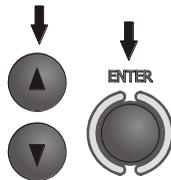
Use ▲, ▼ to switch on/off the function of setting limits, press **ENTER** to confirm.
