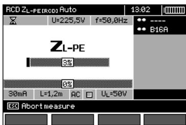
Progress of measurement process is shown by progress bars: bottom - the whole cycle, upper – Z<sub>L-PE</sub> RCD measurement and RCD parameters.
