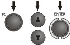
Press **F1** **WIRE** push-button if L lead length needs to be selected. Use ▲ and ▼ to select the lead length and press **ENTER**.
