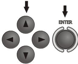
Use **◀**, **▶** and **▲**, **▼** to select the voltage and frequency. Press **ENTER** to select the desired item. Press **F4** (OK) to approve the selection.
