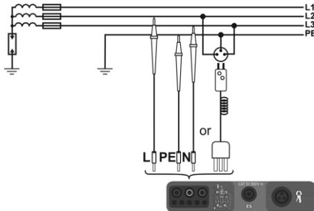
The way of making short circuit loop measurements is described in point 3.4.1. Operating voltage range: 95 V ... 440 V.
