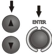
Use ▲, ▼ to select automatic or manual incrementing of field number after entering it to the memory (automatic incrementing is deactivated), press **ENTER** to approve the selection.
