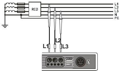
The arrow rotates to the right: correct sequence of phases; the arrow rotates to the left: incorrect sequence of phases.
