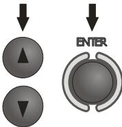
Select  $R_{CONT} \pm 200$  mA item by means of  $\blacktriangle$  and  $\blacktriangledown$  push-buttons and confirm by pressing ENTER.
