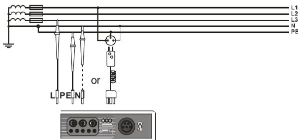
Checking effectiveness of protection against electric shock of the meter housing in case of: a) TN network b) TT network
