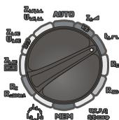
Set the rotary switch of function selection at  $t_A$  position.
