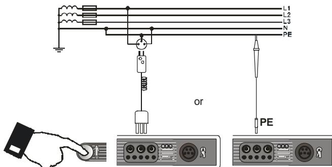
When the meter is connected according to the drawing, touch the touch electrode with a finger and wait for about 1 second. When voltage is found on PE, the device displays **PE!** message (error in the installation; PE lead is connected to the phase lead) and generates a continuous audio signal. This possibility is available for all measuring functions that apply to residual current devices (RCD) and short circuit loop.
