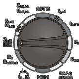
Set the rotary switch of function section at  $Z_{L-PE}$  **RCD** position.
