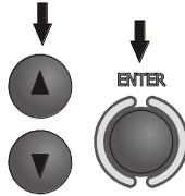
By means of ▲, ▼ push-buttons select the option of automatic incrementing of field number after its storing in the memory or the manual incrementing option (automatic incrementing option (automatic incrementing is deactivated)); confirm a choice made by means of **ENTER** push-button.
