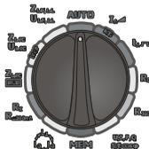
Set the rotary switch of function selection at **AUTO** position.
