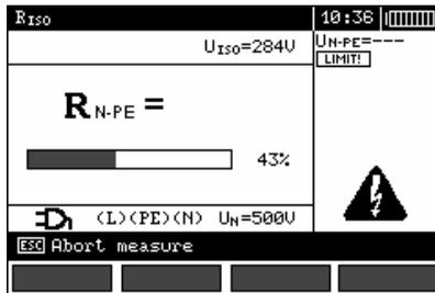
View of the screen during measurement. Symbol of the resistance being measured is displayed. Progress bar shows % of progress of total measurement.
