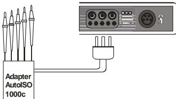
Connect AutoISO-1000c adapter. The meter detects this fact automatically and changes the appearance of the screen.
