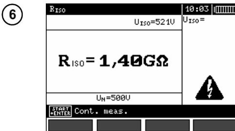
View of the screen during measurement performed with the use of **ENTER** push-button.
