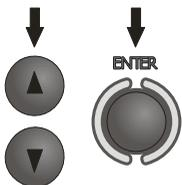
Mark an appropriate position by means of ▲ and ▼ push-buttons and confirm by pressing **ENTER**.
