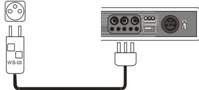
Connect WS-03 lead or WS-04 lead to the socket tested.
