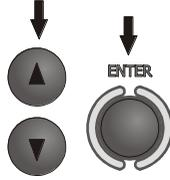
Select a proper item by means of ▲, ▼ push-buttons. Enter a selected option by pressing **ENTER**.
