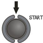
Press **START** push-button in order to start a next measurement without disconnecting test leads from the object.
