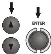
Set the time or deactivate Auto-OFF by means of ▲, ▼ push-buttons; confirm a choice made by means of **ENTER** push-button.
