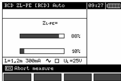
Progress of measurement process is shown by progress bars: lower bar – total cycle; upper bar – measurement of  $Z_{L-PE}$  RCD and  $I_A$ .
