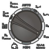
Set the rotary switch of function selection at **R<sub>ISO</sub>** position.
