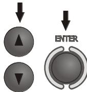
By means of ◀, ▶ push-buttons select a parameter to be changed, by means of ▲, ▼ select network voltage and frequency. Confirm a choice made by means of **ENTER** push-button.
