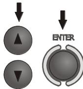
Select contrast value by means of ▲, ▼ push-buttons; confirm a choice made by means of **ENTER** push-button.
