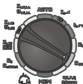
Set the rotary switch of function selection at  $R_{ISO}$  position.
