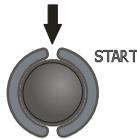
Press **START** push-buttons to start measurement. If any of the voltages exceeds allowable voltage value (50 V), **Object under voltage** message is displayed and the measurement is blocked.
