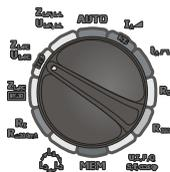
Set the rotary switch of function selection at  $Z_{L-PE}/U_{L-PE}$  position.
