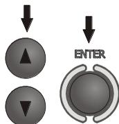
Use the ▲ and ▼ buttons to select the backlight off (with the
