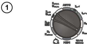
Set the rotary switch of function selection at **R<sub>iso</sub>** position.
