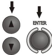
Select a suitable item by means of ▲, ▼ push-buttons; enter the edition of a selected option by means of **ENTER** push-button.
