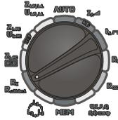
Set the rotary switch of function selection at  $R_X R_{\pm 200}$  mA position.
