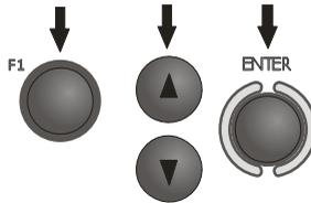
Press **F1** push-button. Select "**U, I, f,  $\cos\varphi$ , P, Q, S**" by means of **▲** and **▼** push-buttons and press **ENTER** push-button. (If you want to measure voltage or current only, select a proper position.)
