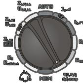
Set the rotary switch of function selection at **U, I, P, Q, S, f,  $\cos\varphi$**  position.
