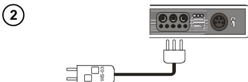
Connect WS-03 lead or WS-04 lead with UNI-Schuko outlet plug. The meter detects this fact automatically and changes the appearance of the screen.
