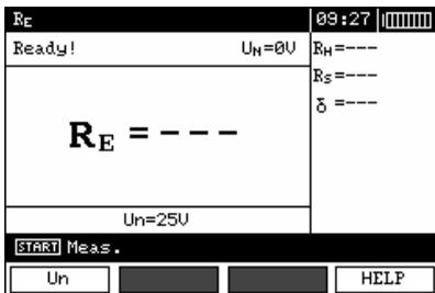
The meter is ready for measurement. Value of interference voltage  $U_N$  can be read on the display.
