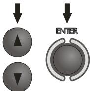
Select an appropriate item by means of ▲ and ▼ push-buttons and confirm by pressing ENTER.
