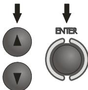
Select test voltage by means of push-buttons and confirm by pressing **ENTER**.
