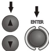
By means of ▲, ▼ push-buttons select main result in the form of impedance  $Z_s$  or prospective short-circuit current  $I_k$ ; confirm a choice made by means of **ENTER** push-button.
