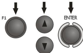
Press **F1** push-button if L lead length needs to be selected. Select a lead length by means of **▲** and **▼** push-buttons and press **ENTER** push-button.
