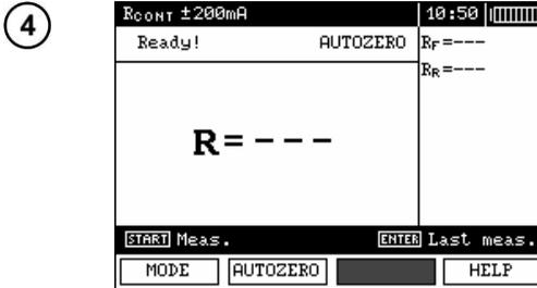
AUTOZERO message appears that confirms completion of test leads calibration.
