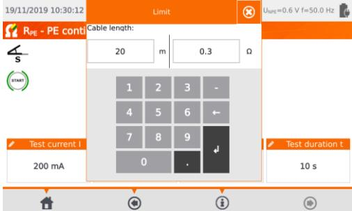
**Resistance limit** resulting from the length of the PE conductor. Use keyboard to enter:
