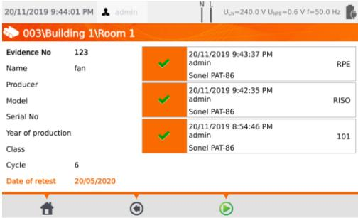
The appliance data (left) and the list of measurements taken (right) are displayed.
