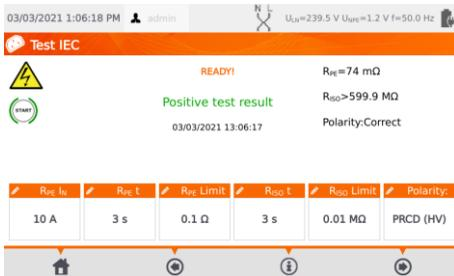
✓ Positive test result: parameters are within limits
