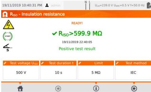
✓ Positive test result:  $R_{ISO} \geq \text{LIMIT}$
