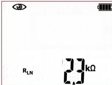
The tester is waiting for the evaluation of the device after completing visual inspection. If the measurement of the L-N circuit resistance is selected, tester will also display the result of  $R_{LN}$  measurement. If it's not selected, then dashes will be displayed in the main screen area „----“.
