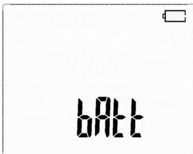
Rechargeable batteries completely discharged.
