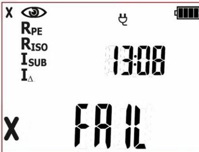
Negative visual inspection result, further measurements will not be conducted. Red LEDs of FAIL indication are on. On the right side of the screen the current time is shown.
