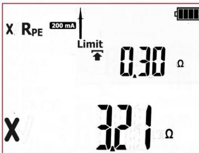
Inorrect result. The value of PE resistance is above the set limit. Red LEDs of FAIL indication are on.
