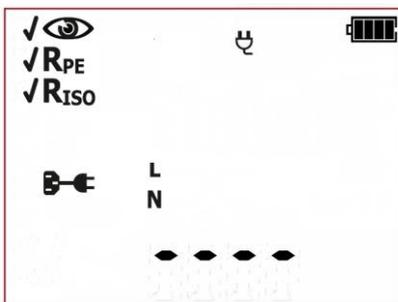
Measurement of insulation resistance has been completed. If the measurement result is negative, further measurements will not be conducted. In case of the positive test result: **the tester will automatically run the subsequent tests – polarity check.**
