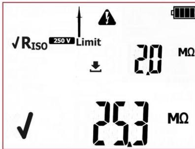
Correct result. The value of insulation resistance is above the set limit. Green LEDs of PASS indication are on.
