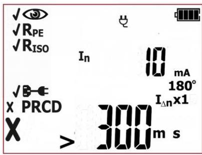
Incorrect result. One or more of the measured parameters are above the permissible threshold. Red LEDs of FAIL indication are on.
