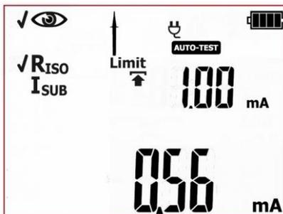
Measurement of  $R_{ISO}$  insulation resistance has been completed. If the measurement result is negative, further measurements will not be conducted. In case of the positive test result: If the **AUTO-TEST** (**AUTO-TEST**) mode is on, the tester will automatically run the subsequent test, which by default is:  $I_{SUB}$ . If the **AUTO-TEST** mode is off the tester will wait for the **START/STOP** button to be pressed. At this stage it is possible to return to the previous test to repeat
