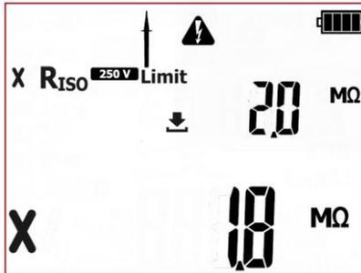
Incorrect result. The value of insulation resistance is below the set limit. Red LEDs of FAIL indication are on.
