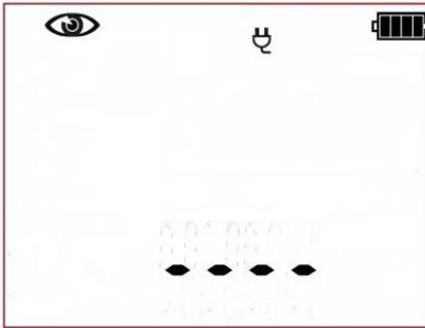
The tester is waiting for the evaluation of the cable's (extension cord) condition after completing visual inspection.
