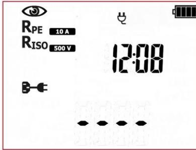
The tester is in IEC testing mode. On the right side the current time is shown.
