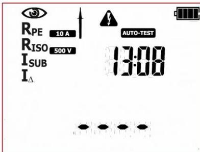
The tester is in autotest mode for Class I devices. Icons displayed on the left side represent all tests that will be performed. On the right side the current time is shown.
