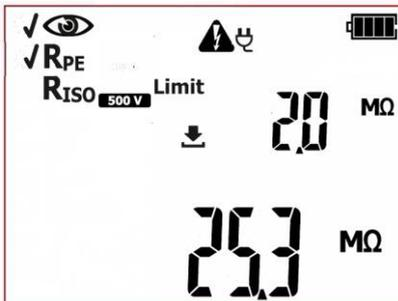
Measurement of PE protective conductor has been completed. If the measurement result is negative, further measurements will not be conducted. In case of the positive test result: **the tester will automatically run the subsequent test: R<sub>ISO</sub>.**
