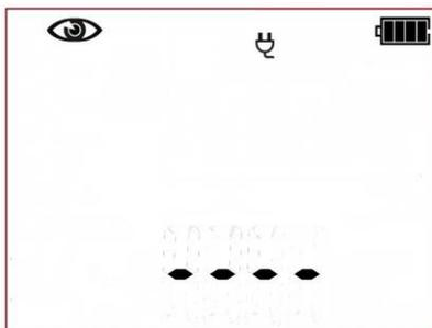
The tester is waiting for the evaluation of the device after completing visual inspection. If the measurement of the L-N circuit resistance is selected, tester will also display the result of  $R_{LN}$  measurement. If it's not selected, then dashes will be displayed in the main screen area „----”.
