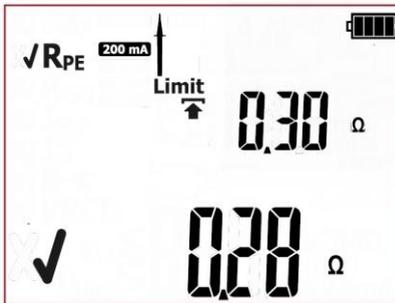
Correct result. The value of PE resistance is below the set limit. Green LEDs of PASS indication are on.
