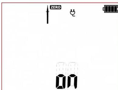
The compensation value has been measured.  $\Omega$  is displayed on the screen, along with the permanent **ZERO** symbol. After 3 seconds the tester returns to measurement mode. The active test lead compensation is indicated by **ZERO** icon being displayed on screen during the tests of  $R_{PE}$  (200mA, 10A) and CL I autotests. The compensation resistance will be taken into account then displaying test results of  $R_{PE}$ .
