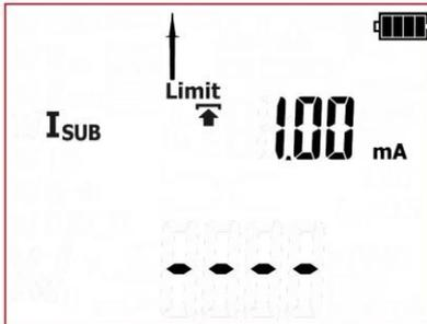
The tester is in substitute leakage current measurement mode.
