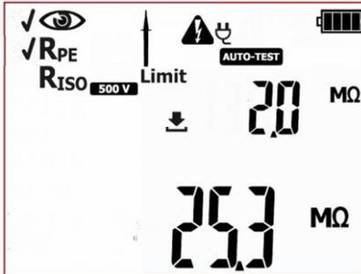
Measurement of PE protective conductor has been completed. If the measurement result is negative, further measurements will not be conducted. In case of the positive test result: If the **AUTO-TEST** mode is on, the tester will automatically run the subsequent test, which by default is: **R<sub>ISO</sub>**. If the **AUTO-TEST** mode is off the tester will wait for the **START/STOP** button to be pressed. At this stage it is possible to return to the previous test to repeat
