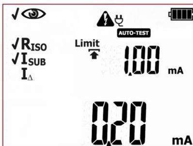
Measurement of substitute leakage current has been completed. If the measurement result is negative, further measurements will not be conducted. In case of the positive test result: If the **AUTO-TEST** (**AUTO-TEST**) mode is on, the tester will automatically run the subsequent tests. If the **AUTO-TEST** mode is off the tester will wait for the **START/STOP** button to be pressed. At this stage it is possible to return to the previous test to repeat
