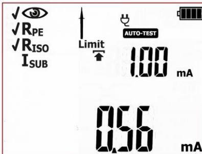
Measurement of insulation resistance has been completed. If the measurement result is negative, further measurements will not be conducted. In case of the positive test result: If the **AUTO-TEST**
