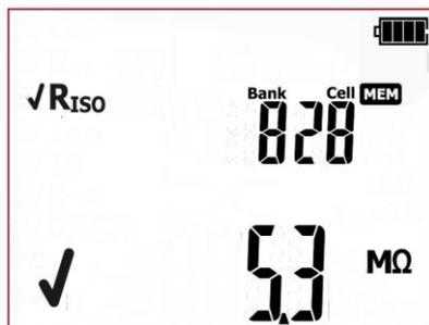
A cell occupied by a single test result. An icon indicating the test type and the main result is displayed on screen.
