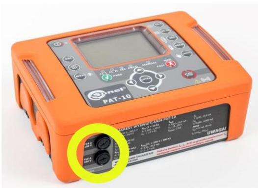
The next step is to replace the fuse with a new one and fit it together with its container back into the tester.
