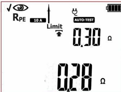
Positive visual inspection result. If the **AUTO-TEST (AUTO-TEST)** mode is on, the tester will automatically run the subsequent tests, which by default is: R<sub>PE</sub>. If the **AUTO-TEST** mode is off the tester will wait for the **START/STOP** button to be pressed.
