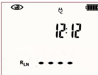
The tester is now in the preliminary test-visual inspection mode. Additionally the current time is displayed on the screen.
