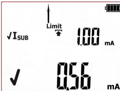
Correct result. The value of leakage current is below the set limit. Green LEDs of PASS indication are on.
