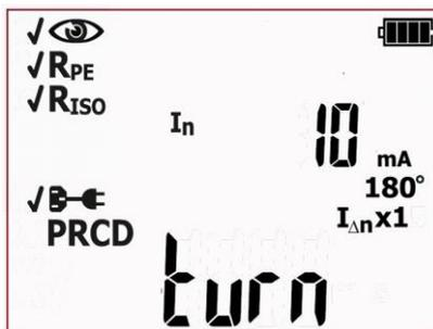
Switch on PRCD. Tester will commence the first measurement. If PRCD trips, a message prompting to switch on the RCD will be displayed on the main screen: **'turn on PRCD'**.
